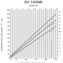
SYSTEM SUPPLY PRESSURE - PSI  $\longrightarrow$  EQUIVALENT LENGTH BASED ON 1/2" SCHEDULE 40 PIPE WITH C=120
