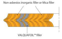
By winding VALQUAFOIL™ filler in the middle of inorganic fillers, these spiral Wound Gaskets have enhanced gas sealability with increased compatibility with flanges. Further, the inner filler and outer filler shuts off the oxygen supply, inhibiting the oxidation of VALQUAFOIL™ under oxidizing conditions and makes it possible to be used in high temperatures.
