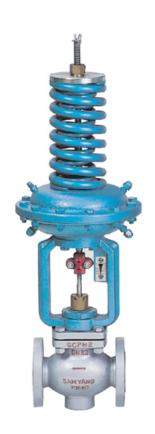
As a Pressure reducing valve for high pressure fluids with diaphragm on its pressure detecting part, it guarantees stable operation at large differential pressure across the disc. And the adoption of pressure balance construction assures good regulation of pressure management at the secondary side regardless of the variance at the primary size.
