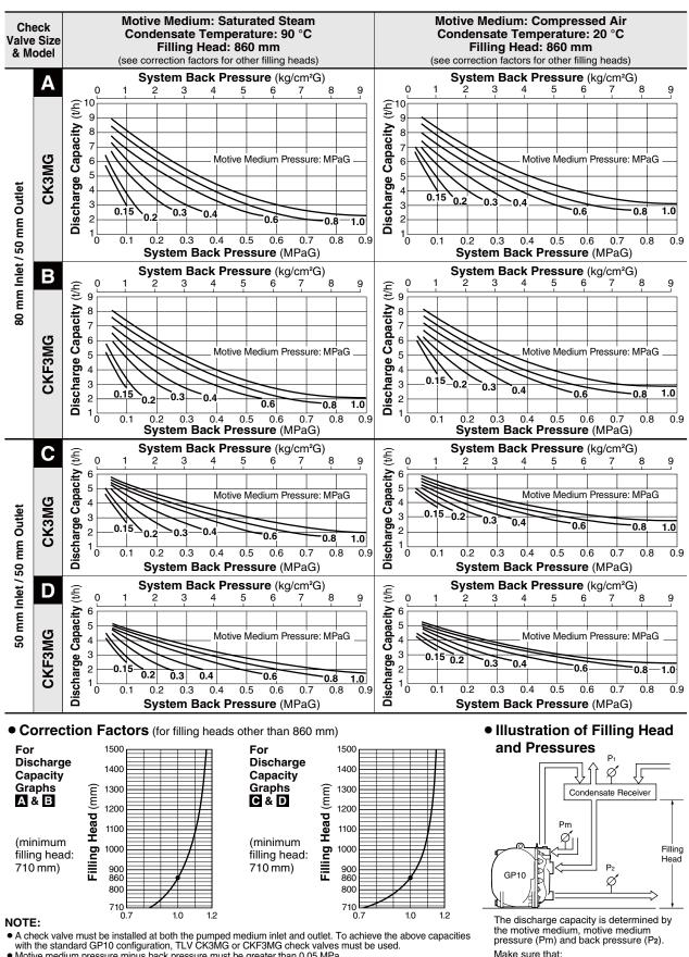
A check valve must be installed at both the pumped medium inlet and outlet. To achieve the above capacities with the standard GP10 configuration, TLV CK3MG or CKF3MG check valves must be used.
