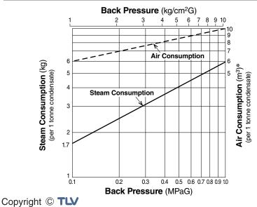
\* Equivalent consumption of air at 20 °C under atmospheric pressure
