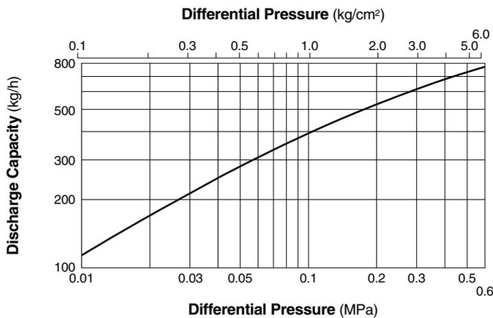
1. Differential pressure is the difference between the inlet and outlet pressure of the trap.
