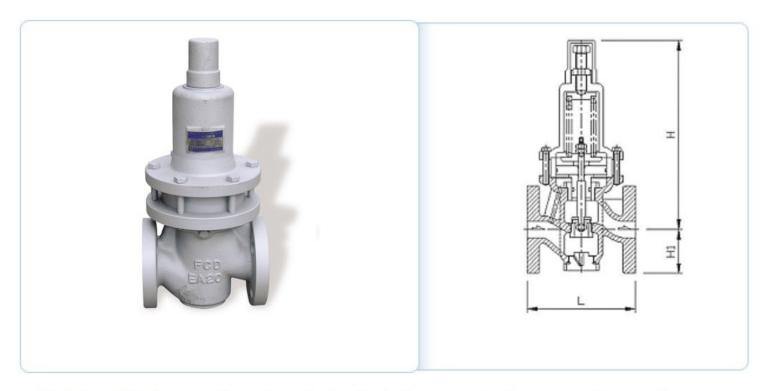
A kind of a relief valve or a self-actuating adjustment valve for maintaining the pressure of instruments or pipelines by exhausting excessive pressure according to load variation. This is widely used for a valve for adjusting the pressure of cold or warm water in an air conditioning or a heating/cooling facility of medium- and high-rise buildings.
